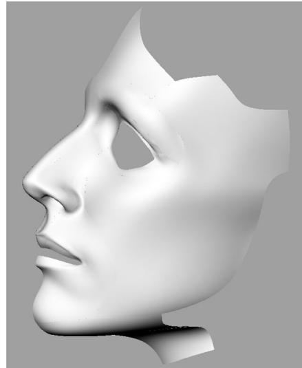
After having transferred the faces you are able to use Rhinos face evaluation tools to check the output. If some problems occur, please try to modify the poly lines by moving the points or adding new poly lines.
